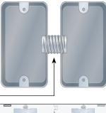
Two single-gang backboxes connected by a chase nipple with 3/4 in separation.
