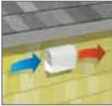
Supply and exhaust air flows through a single exterior opening
